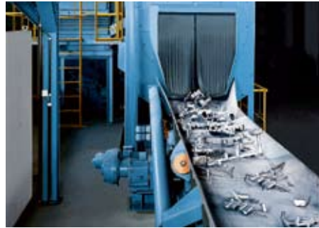
Exit side with stepped chute and abrasive return
