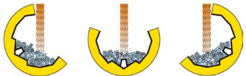
Rocking motion of the polygon-shaped trough about its longitudinal axis for gentle tumbling of the castings
