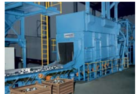
The DT 14 throughfeed blast cleaning machine for economical, low-pollution, non-hazardous operation
