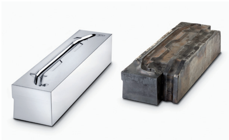
Cleaned and reconditioned forge tool
